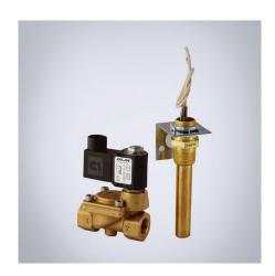
**Description:** Brass solenoid valve and thermostat that limit the flow of compressed air to only when cooling is needed. The thermostat is factory set at 35 °C, but adjustable to any other temperature. The thermostat mounts in a 22 mm diameter hole, and it may be mounted through the enclosure wall or on a bracket inside the enclosure. The thermostatically controlled vortex cooler saves compressed air, and it is recommended where heat load fluctuates and continual purge is not required.
