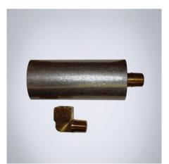
**Description:** To reduce the noise from the vortex cooler. It mounts directly to the nozzle of the vortex cooler, inside the enclosure. It reduces around 15% the vortex cooler noise.
