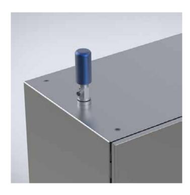
This Vortex cooler, BP, with a IP 66 protection degree, is easy to install, has no moving parts, and is maintenance free. In addition to cooling, it also reduces the relative humidity within the enclosure it is mounted on. This Vortex cooler is an ideal solution to prevent overheating within the enclosure.
