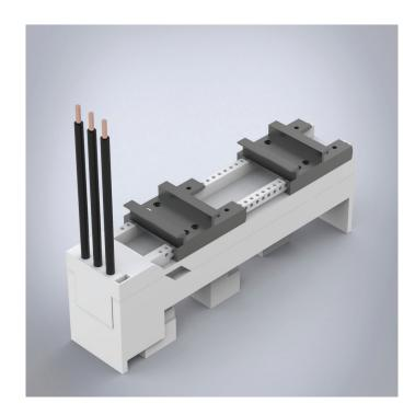
**Description:** Busbar adapter 25 A. With two adjustable mounting rails. With removable upper section and leads (4  $\rm mm^2$ ).
