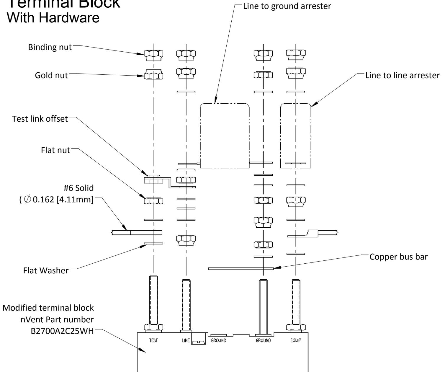
1. Assemble all hardware, test link, arrestors, and wires as shown.
