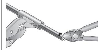
Continue this motion in a series of short "rips", keeping the side cutters at about 45° to the line of the cable, removing sheath spirally. Remove compacted powder insulation to expose conductors.
