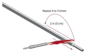
It may be necessary to repeat the above procedure several times to completely remove all moisture from the cable. Allow the cable to cool before repeating. On completion, check IR with a 500-V insulation tester (Megohmmeter).
