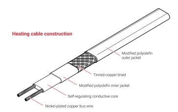
The nVent RAYCHEM WFP-612 and WFP-622 heating cables are specifically designed for use with nVent RAYCHEM RIM2 panels, providing energy efficient solution for moderate snow load areas.
