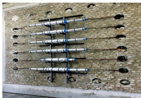
Figure 4. UL 2196 Cable Test Wall
