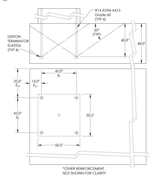
Note that the anchors in this example meet the definition of an anchor group (defined as "a number of similar anchors having approximately equal effective embedment depths with spacing between adjacent anchors such that the projected areas overlap," reference Section 2.3 of ACI 318-14 (Section D.1 of ACI 318-11)). Furthermore, due to the proximity to edges, additional factors must be considered compared to Example B1 in this design aid.
