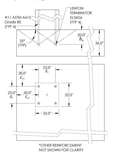
Concrete Breakout Strength in Tension of a Single Anchor ( $N_{cb}$ ): Breakout strength in tension can be calculated for a single anchor with the equation found in Section 17.4.2.1a of ACI 318-14 (D.5.2.1a of ACI 318-11).
