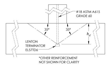
Evaluating the headed rebar to Chapter 17 of ACI 318-14 (Appendix D of ACI 318-11) enables the calculation of concrete breakout strength in tension  $(N_{ch})$ , pullout strength in tension  $(N_{pn})$ , and concrete side-face blowout strength in tension  $(N_{sh})$  to ensure that the designed performance meets the factored tensile force  $(N_{ua})$ , which in this case is 240,000 lbf.
