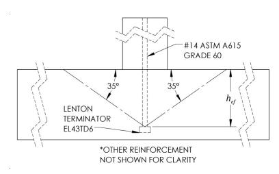
Evaluating the headed rebar to Chapter 17 of ACI 318-14 (Appendix D of ACI 318-11) enables the calculation of concrete breakout strength in tension  $(N_{ch})$ , pullout strength in tension  $(N_{pn})$ , and concrete side-face blowout strength in tension  $(N_{sh})$  to ensure that the designed performance meets the factored tensile force  $(N_{ua})$ , which in this case is 135,000 lbf.
