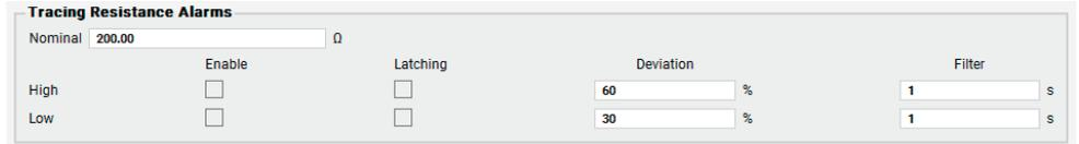
The image shows a configuration window titled "Tracing Resistance Alarms". It features a "Nominal" value of 200.00 Ω. Below this, there are two rows for "High" and "Low" deviation settings. Each row includes an "Enable" checkbox, a "Latching" checkbox, a "Deviation" percentage input field, and a "Filter" input field. The "High" row has a deviation of 60% and a filter of 1. The "Low" row has a deviation of 30% and a filter of 1.
