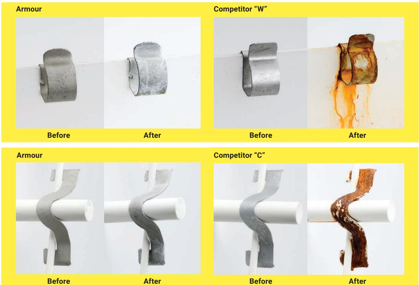
\* Salt-spray testing test method: ASTM B117 / DIN 50021; Cyclic corrosion test method: GM 9540P. See <https://www.nvent.com/our-brands/CADDY> for the terms of the Armour 10-year limited warranty.
