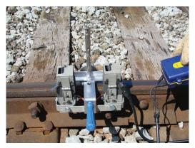
Press and hold control unit switch and wait for the ignition.
