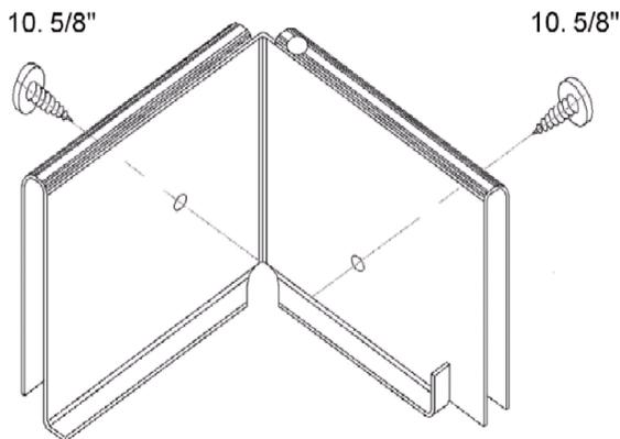
The CADDY® SFCLT is designed to work together with the T-Bar runners to provide seismic restraint for the fixture. It is essential to install each CADDY SFCLT using 2 #10 self-tapping screws provided in the package. All four clamps must be installed on each fixture.
