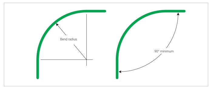
Figure 11: Bend Radius on TEBC Conductor
