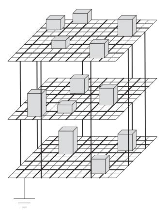
Figure 6: Mesh Bonded Network TIA 607 C
