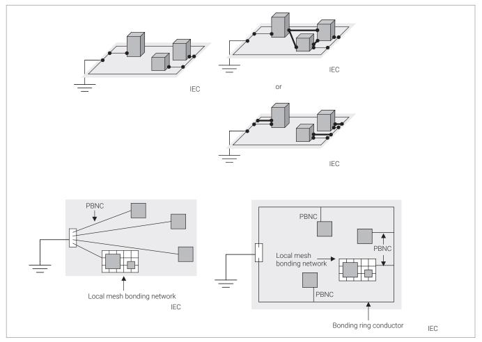
Figure 8: Additional Bonding and Localized Mesh Networks IEC30129
