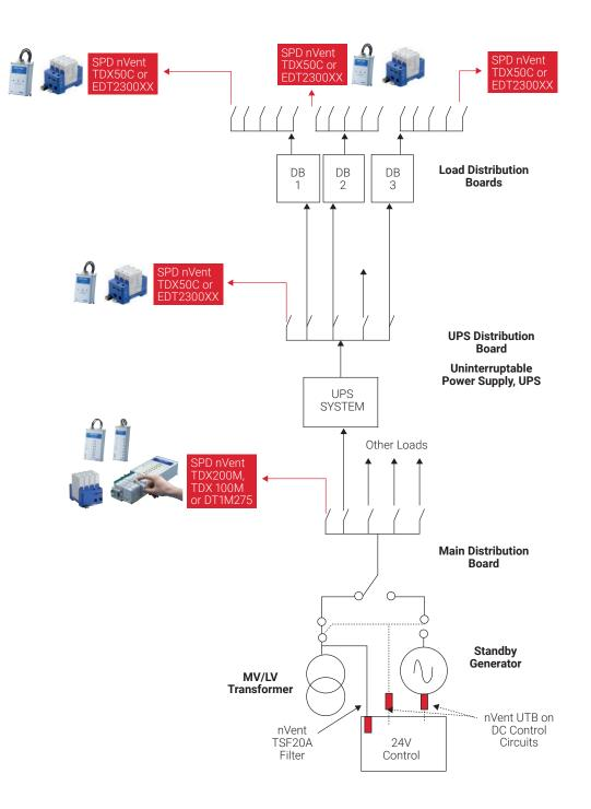
Figure 18: Surge Protection Scheme at a Data Center - Line Diagram
