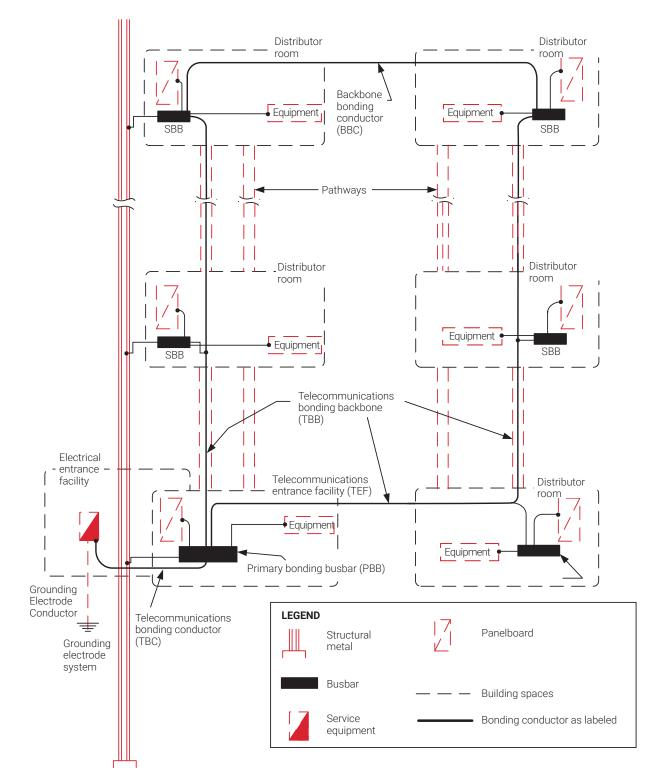
The PBB also serves as the central attachment point for the Telecommunication bonding backbone TBB, Secondary bonding bars, SBB and equipment. Telecommunications bonding conductor (TBC) bonds the PBB to the service equipment (power) ground.
