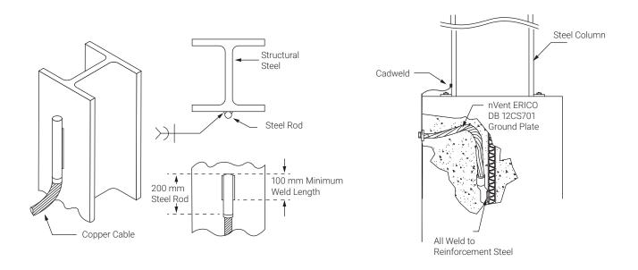
Figure 14: Ground Electrode- Building with Basement
