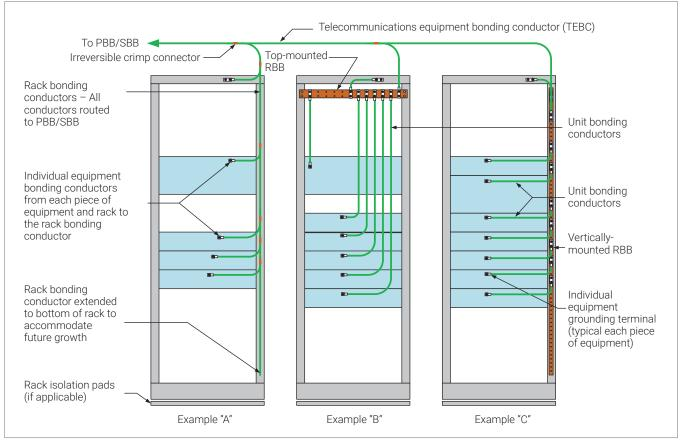
Figure 9: Equipment & Cabinet Bonding
