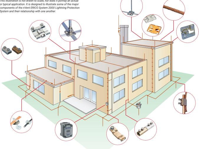
Figure 20: nVent ERICO System 2000 or Conventional Lightning Protection System
