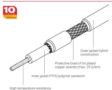
nVent RAYCHEM XPI-F is a polymer insulated (PI) series heating cable, suitable for use in ordinary and hazardous areas. It has been designed for freeze protection and low temperature maintenance applications on pipes, tanks and other equipment.
