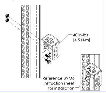
2) Fasten support rails to bracket using M10 Hex Bolt and M10 Hex Nut. Reference instruction sheet IP8347 for CABS system installation.
