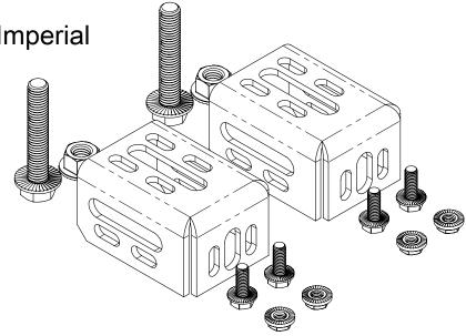
1) Attach bracket to enclosure frame in the desired orientation using M6 Hex Bolts and M6 Hex Nuts. Alternative: Use two (2) cage nuts instead of hex nuts (not included) OR two (2) Hoffman BVM6 fasteners (not included).
