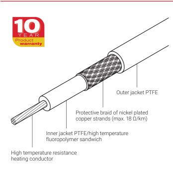
nVent RAYCHEM XPI is a polymer insulated (PI) series heating cable, suitable for use in hazardous areas. It has been designed for use in freeze protection and temperature maintenance applications of pipes, tanks and other equipment. XPI offers an economical solution for a wide variety of heat-tracing applications, in particular for pipe lengths beyond the maximum circuit lengths of parallel heating cables.
