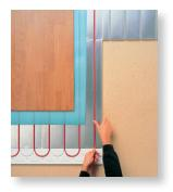
In the en-suite bathrooms, high-powered T2Quicknet 160, a thin self-adhesive heating mat, was used as it provides fast heat up time and at only 3mm thick proved ideal for installation under the tiled floors with the additional benefit that they not only heat but also dry the floors to prevent slipping. These same mats were also installed in the hotel's luxurious spa in conjunction with RAYCHEM T2 Isolecta insulation board, to offer an energy efficient, smart solution.
