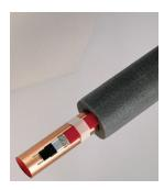
RAYCHEM HWAT are self-regulating heating cables that adjust their power output to compensate for variations in water and ambient temperatures. They replace supply-pipe heat losses at the point where the heat loss occurs, providing continuous, energy-efficient hot water temperature maintenance and eliminating the need for a recirculation system.
