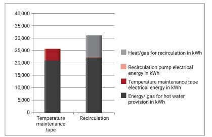
Fig. 4: Useful energy consumption of the condensing heat generator with primary cylinder for hot water provision and heat loss compensation of the pipes with temperature maintenance tape or recirculation pipe.
