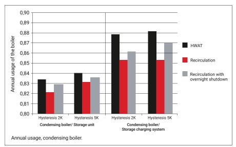
Fig: 2 Annual level of use the condensing boiler.
