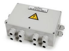
The nVent RAYCHEM RMM2 Remote Monitoring Module provides up to eight additional resistance temperature detectors (RTDs) to measure additional temperatures for control and monitoring of the heat-tracing circuits. Multiple RMM2s communicate with a single UIT to provide centralised monitoring of temperatures.
