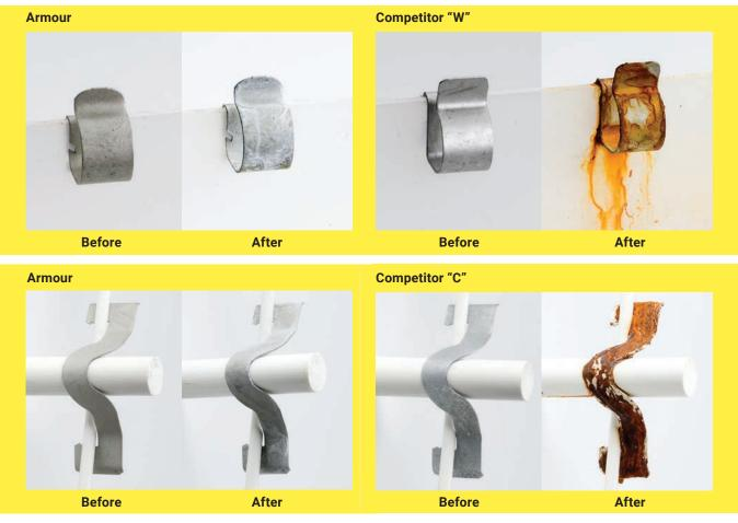
\* Salt-spray testing test method: ASTM B117 / DIN 50021; Cyclic corrosion test method: GM 9540P. See https://www.nvent.com/our-brands/CADDY for the terms of the Armour 10-year limited warranty.
