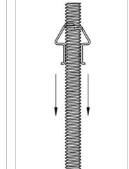
When the threaded rod is no longer pushed or is pulled, thanks for the nature of spring steel, the flexing arms go back to their initial position instantly locking the threaded rod in place
