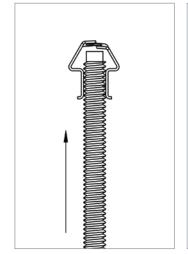
Threaded rod enters the housing and pushes against the two flexing arms
