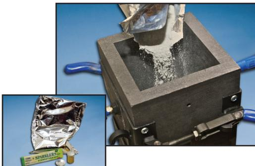
Cadweld welding material is a mixture of copper, aluminum and other ingredients. Each bag or container contains sufficient welding material for the specified connection. Cadweld welding material cannot ignite spontaneously. It can be handled and stored without danger. Adding starting material to the welding material is necessary to begin the exothermic reaction.
