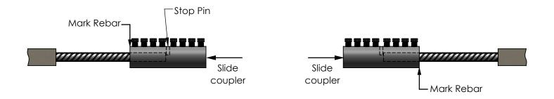
Step 2: To allow rebar to pass entirely through the coupler, remove the stop pin by pushing the pin into the inside diameter of sleeve. Discard the stop pin.
