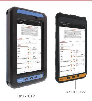
The Ecom Tab-Ex 03 is an easy-to-use wireless tablet for configuration and monitoring of nVent RAYCHEM NGC-20 and Elexant 5010i field controllers. The tablet has an intuitive user interface eliminating the need for extensive training. The tablet is available in two versions: For Zone 2 (Zone 22) use the Tab-EX 03 DZ2. For Zone 1 (Zone 21) use the Tab-Ex 03 DZ1.
