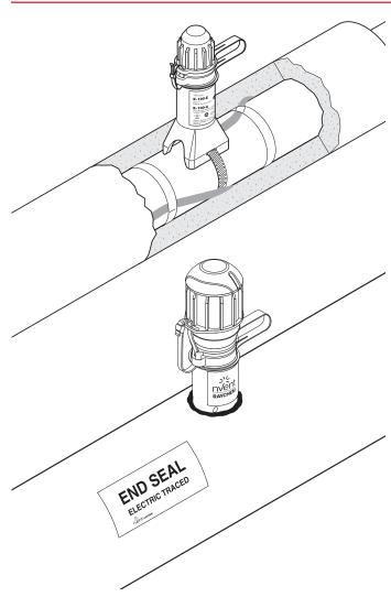
Both the nVent RAYCHEM E-100-E and E-100-L-E are accessible, re-entrable end seals, the E-100-E without a light, the E-100-L-E with a signal light. Both end seals can be used with all nVent RAYCHEM BTV, QTVR, XTVR, HTV or VPL industrial parallel heating cables. They are approved for use in hazardous areas. They are extremely rugged - made of a strong, moulded part with 4 mm wall thickness.
