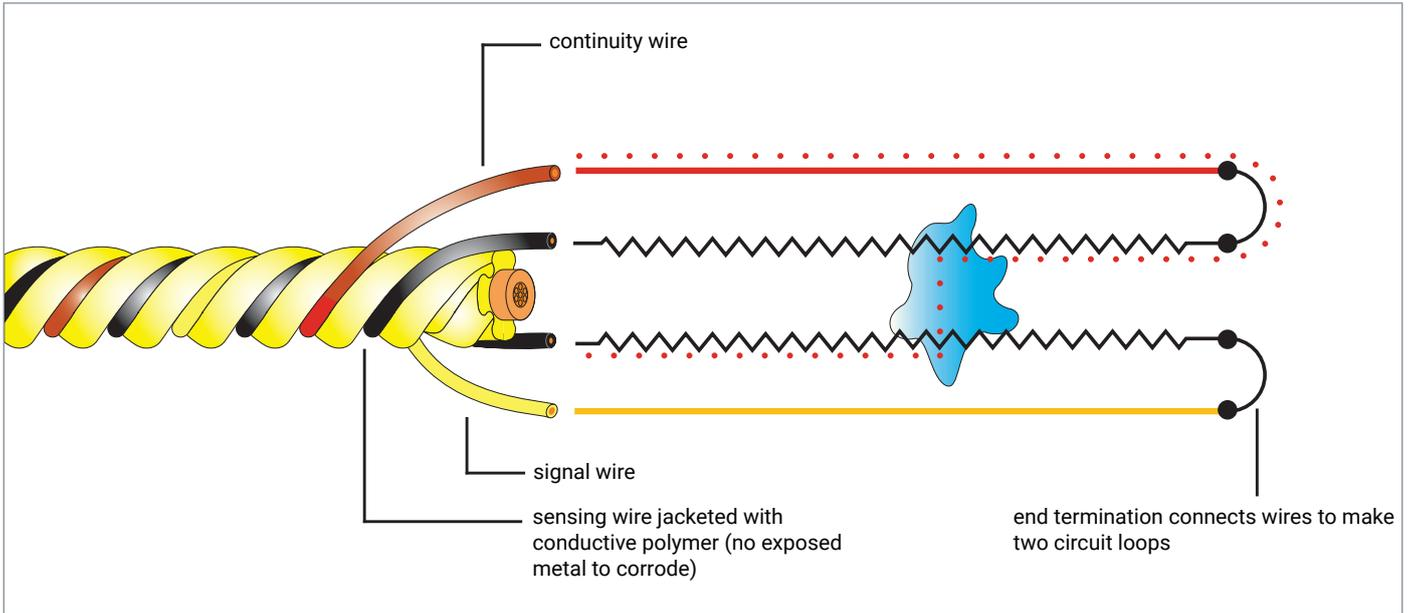
Conductive polymers are used to extend the life of TraceTek cables. Some of the oldest TraceTek water detection cables have been in continuous service for more than 25 years.
