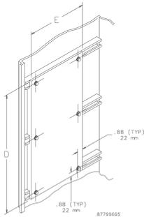
A30S4E Side Mounting Plate used in enclosures, provide a convenient way to install controls and instruments in enclosure body opening while providing access and security.
